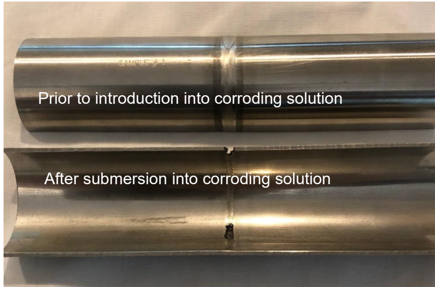
MaxCore 6Mo orbital welded to MaxCore 6Mo with no weld insert
